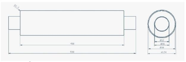
120  $g/m^2$  Aluminium -coated Steel sheet at DX53 degree of hardness
